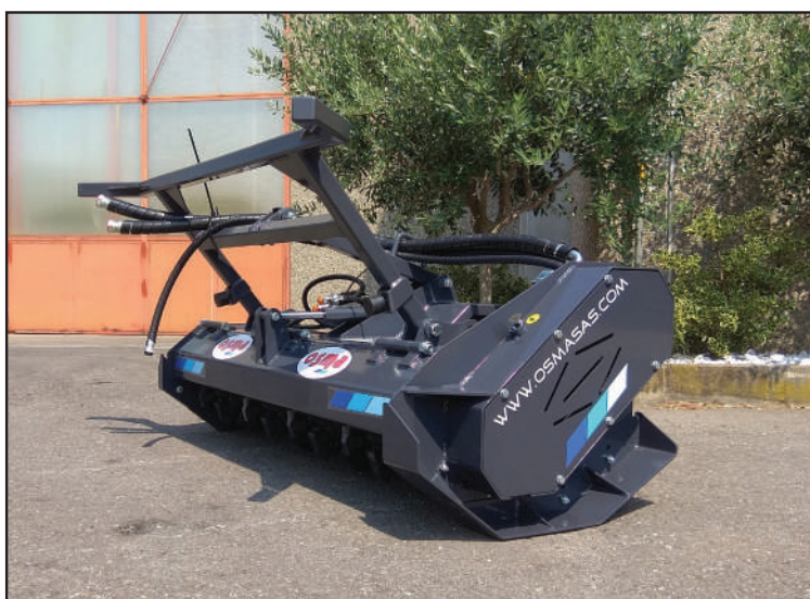
rotor built with 12,5 mm tick tube, internal cover plate in Hardox 400 5mm tick. Under plate skids in Hardox DCR limiter rotor.
