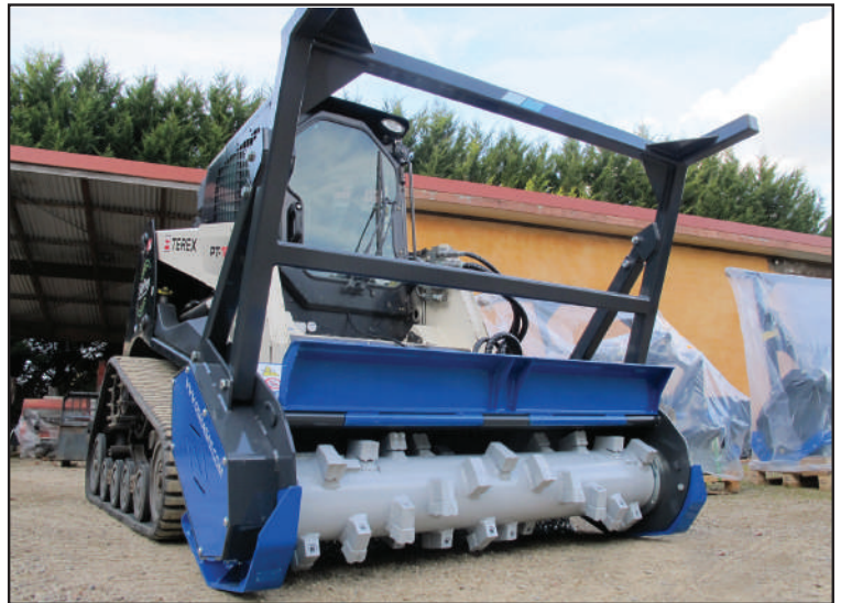
Single drive (4 belts) XPB, steel frame with high tensile limit. Reversible tools (double lifecycle) 3F - OSMA Valve - 1- bypass 2- antishock 3- oil flow automatic regulation.
