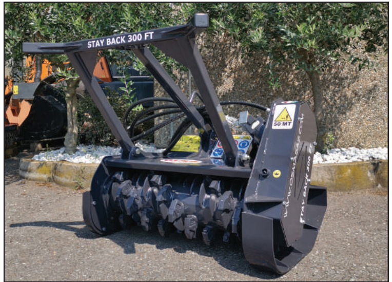
mm tick tube, internal cover plate in Hardox 400 5mm tick. Under plate skids in Hardox, 3F - OSMA Valve - 1- bypass 2- antishock 3- oil flow automatic regulation. Pushing frame
