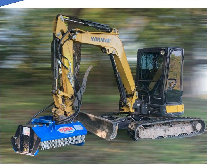
EXH flail Series is designed for 5.5-10 ton excavators to cut dense vegetation and standing material up to 4inches. The EXH has been introduced to the North American market for customers that want to accomplish land clearing and vegetation removal without the need of a fixed tool rotor.
