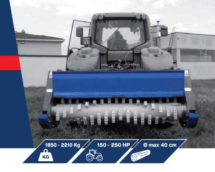
Forestry mulcher Heavy Duty series, drum rotor with fixed Tools, to cut branches, bushes and small trees up to diameter of 40 cms. Tractor power required: from 150 to 250 HP.
