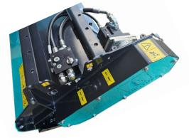
Flow Management combined with CASAPPA Gr.3 Gear Motor without the need of a Case Drain
